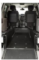
**Option 2 – Second Row Tip & Fold Bucket Seats** Fits one driver, two wheelchair passengers, and three additional passengers
