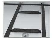
Nylon Casket Rollers — Each deck includes four casket rollers to make moving caskets and air trays in and out of the van easier.
