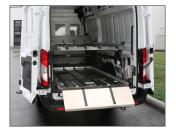
Powered Upper Deck — The upper deck raises and lowers within seconds, allowing one person to easily load and transport cots, caskets, or air trays.
