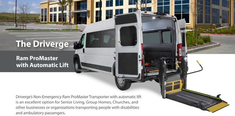
This ADA-compliant Wheelchair-Accessible Ram ProMaster 2500 is equipped with an automatic lift for easy wheelchair access. It is available in Rear-Entry and Side-Entry conversions on 236" length and 102.1" high roof chassis. The Ram ProMaster is designed to cater to both wheelchair-bound and ambulatory passengers.
